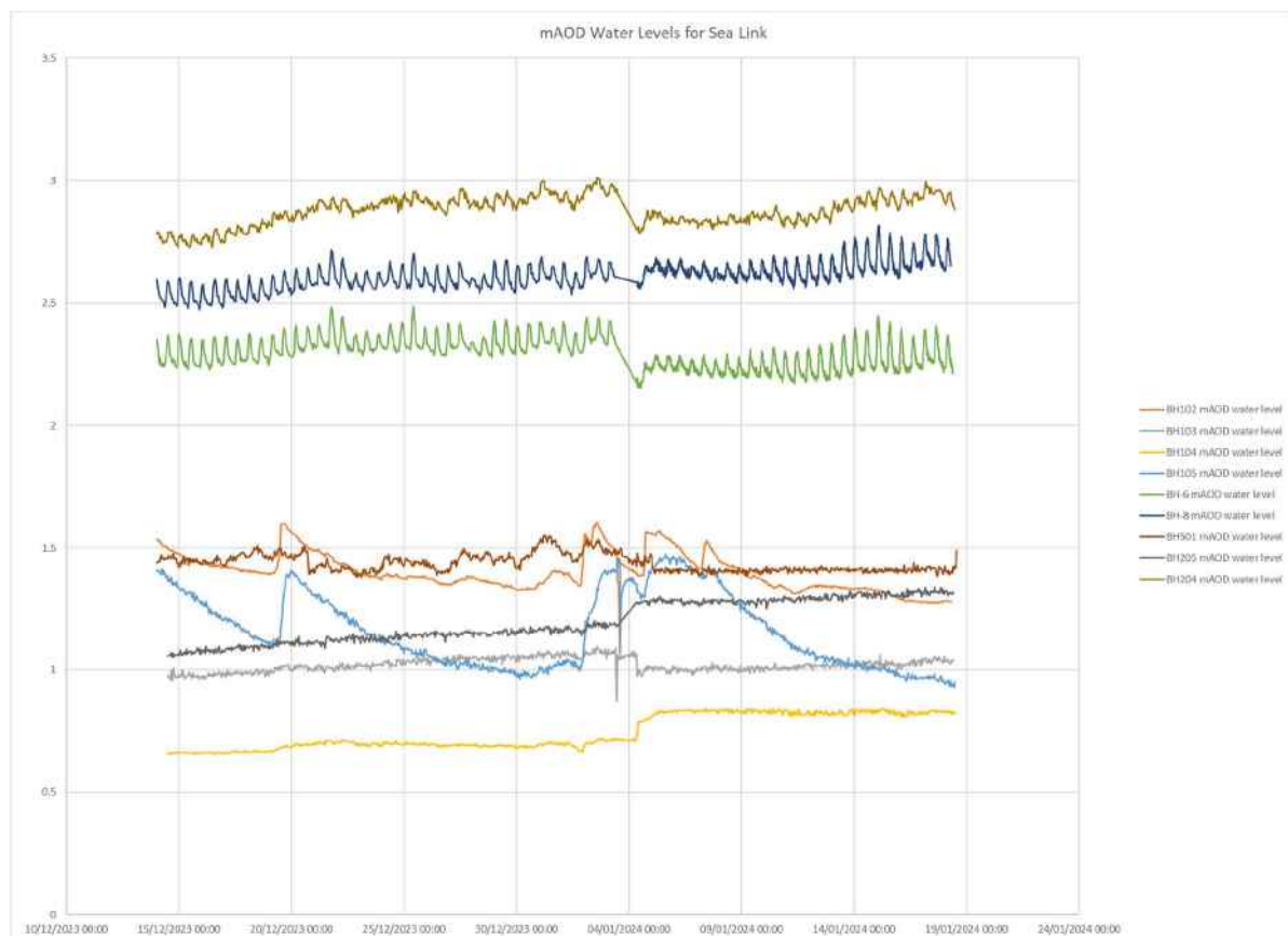
Figure 3 – mAOD elevation plots of boreholes provided.
